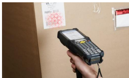
Receive products in using wireless handheld terminals.
